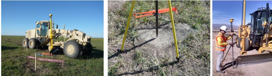
1. Move machine to **Bench Point** with the **Blade low to the ground**
